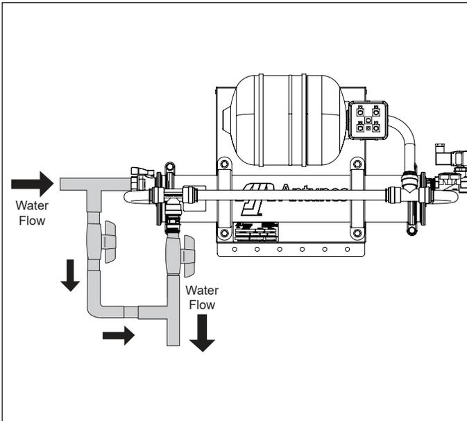
Figure 6. Install Bypass
